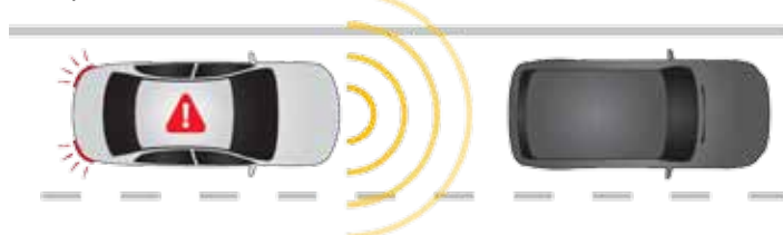
This graphic supplied by ANCAP shows how autonomous emergency braking works
